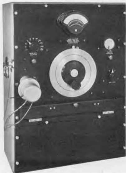
FIGURE 4. Showing the rectifier plugged into the input terminals of a TYPE 636-A Wave Analyzer
