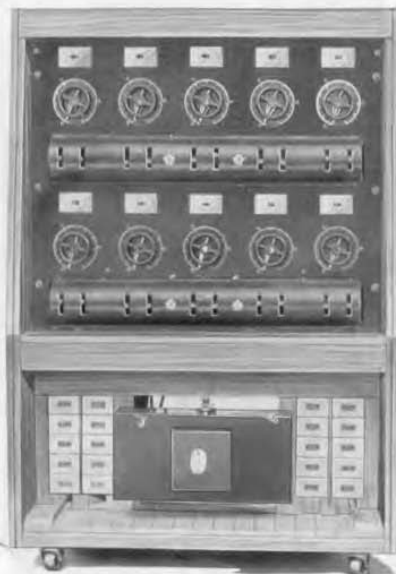
FIGURE 1. Photograph of the lighting-control panel
