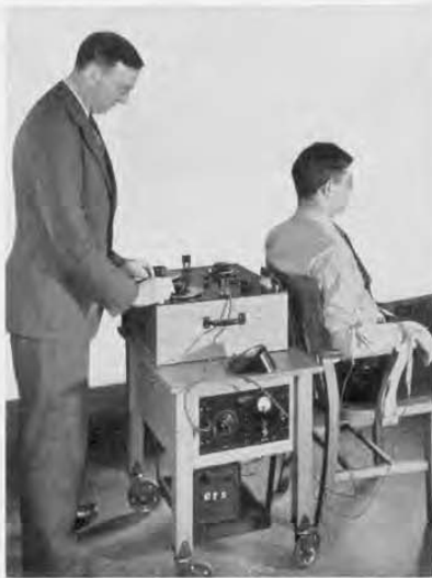
FIGURE 4. For convenience the impedance comparator and its associated amplifier and power supply are mounted on a "tea wagon." The author is shown measuring the impedance of a patient. On the patient's right arm are one inner and one outer electrode. The other pair of electrodes are on the left arm
